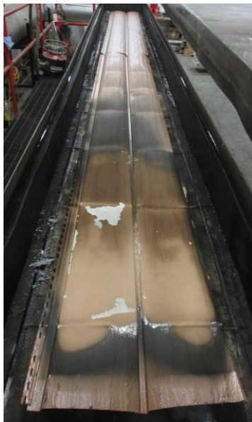
Photo No. 4 Exposed Surface of the Test Specimen (Post-test)
